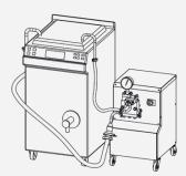
Once the product in the pasteurizer reaches the temperature of 50°C and the sugar has been fully solubilized, the homogenizer starts recirculating the batch in a loop (5 times approx), to make sure the ice cream is fully homogenized.
