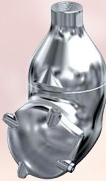
The Bio 10 rotary jet head is a hygienic tank cleaning machine that provides 360deg coverage within a given tank or process vessel. It is self powered by the flow of the fluid through the inlet cone of the machine. An increase in pressure and flow will correspondingly increase the length of the jet and impact upon the tank or vessel surfaces.
